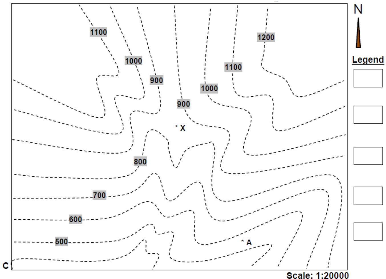
In this map, the lower boundary of limestone bed is exposed out at the elevation of 1050 m. This limestone overlying the shale bed (thickness 150 m). The lower boundary of sandstone bed, which is deposited under this shale bed, is exposed out at the elevation of 700 m. Point A represents the contact between lower boundary of marl bed, which is covered by the sandstone bed, and upperboundary of dolostone bed, which is covered the remained area on the map. The beds are horizontal.
