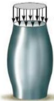
Compression causes material to bulge out (b)
