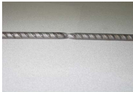
Necking of the rebar before fracture
