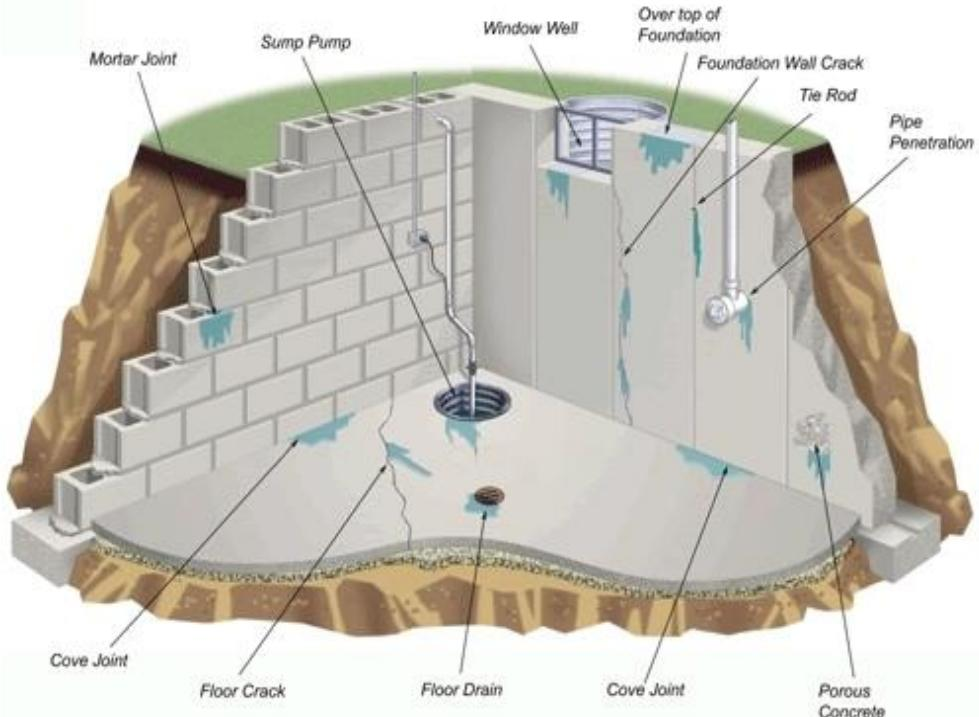
Water can find its way into a basement in many different ways. As this diagram shows, it is possible for water to come through foundation walls, basement wall cracks, and even up from under the basement floor.
